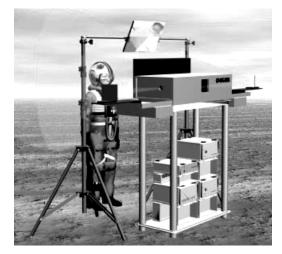
Figure 3. GP-Mini Portable Holography Camera System
